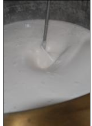
A photo showing a proper vortex is superior to any attempt to define a vortex in writing to someone new to manufacturing—Visual is better!
