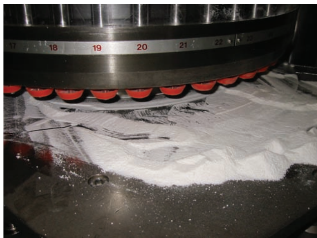
Removing the feeder reveals that too much powder remains on the turret, which leads to overworking the powder and an increase in fines.
