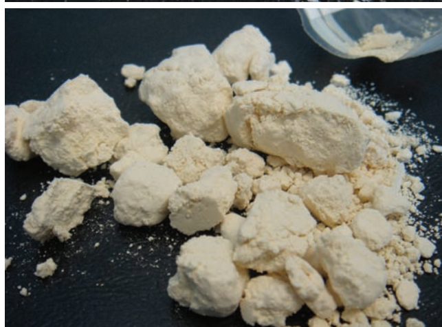
Powders that form lumps make tableting a real challenge. Also, inconsistent powders make inconsistent tablets.
